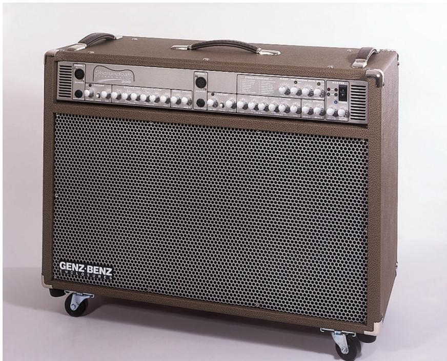
**PRODUCT DESCRIPTION** – The **Shenandoah Stereo Delux 200** is a 2 channel – 4 input, 200 watt true stereo acoustic instrument amplifier with 2 separate Alesis<sup>™</sup> digital effects engines, full stereo DSP algorithms and 2 x 10" speakers and compression tweeters on our unique flexed baffle.
